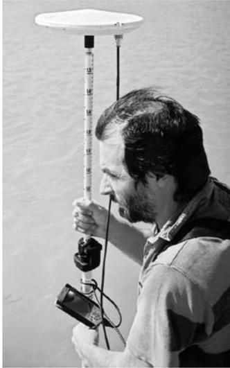
Figure 3: GPS antenna and palmtop
